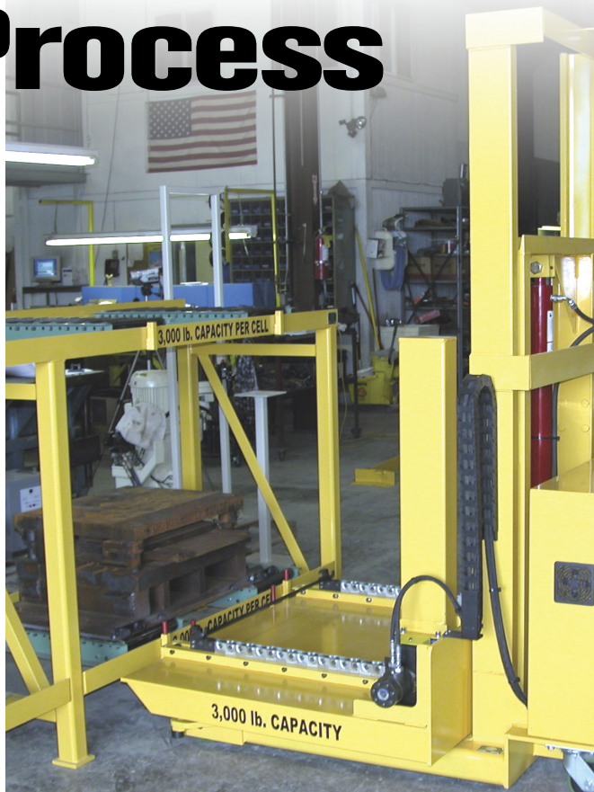
A good first step to quickening the pace of die changes: create an efficient press-room layout, and store dies close and convenient to the press area, with easy access to the dies by the transport vehicle. Photo courtesy of Green Valley Mfg.
